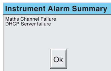
Figure 3.1.4b Typical Instrument alarm summary display
